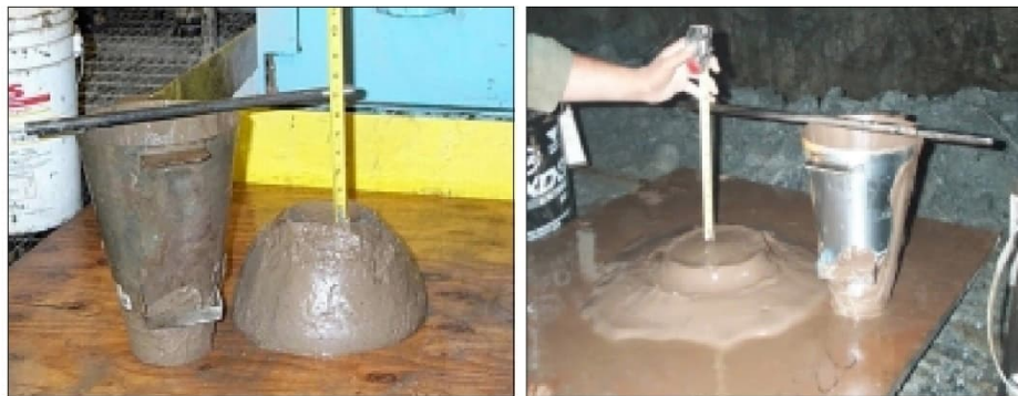
Figure 4-9: Example Slump Tests on Paste (left) and Thickened (right) Tailings Samples
